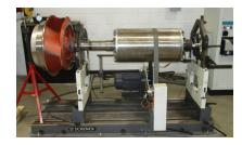
After assembly, the pump is air tested at 6 PSI for one hour then test run and checked for AMP draw, phase balance, and vibration. The pump is then coated with an epoxy based paint.
