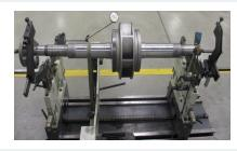
Once our processes are complete, all components undergo a final cleaning and quality control inspection. This process verifies that precision fits, running clearances, and shaft straightness meet or exceed OEM specifications. A careful assembly addresses radial and axial impeller position, thrust, and free rotation.
