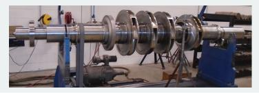
A careful assembly verifies precise impeller centralization at each stage. Our test stand confirms free rotation. These projects involve meticulous details. Our skilled technicians can team up with your staff for final assembly.
