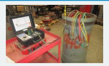
The stator is then baked in our dedicated bake out oven for a minimum of two hours at 250°F. This removes all moisture from the windings and insulation. After this process, the stator will be tested to guidelines listed above.
