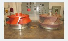
After the rotating assembly is constructed with all components, total indicator runout is verified at less than .003" on critical faces and diameters. The rotor is then dynamically balanced to 4W/N. Our balance stand has a sensitivity of 20 microinches and a capacity of 10,000 lbs.
