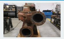
Cleaning consists of a spherical crowned glass bead blast on cast components in our 30' blast booth. Bearing housings are pressure washed and shafting is polished with 400 grit emery cloth. This process allows us to easily spot mechanical wear and erosion in the volute, impeller and shaft.
