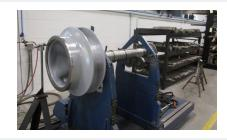
After our processes are complete, all components undergo a final cleaning, hydro test and quality control inspection. This process verifies that precision fits, running clearances, and shaft straightness meet or exceed OEM specifications. A careful assembly addresses radial and axial impeller position, thrust, and free rotation.
