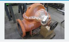
Cleaning consists of a spherical crowned glass bead blast on fabricated and cast components in our 30' blast booth. Bearing housings are pressure washed, and shafting is polished with 400 grit emery cloth. This process prepares all surfaces for an accurate inspection, and allows us to easily spot defects.
