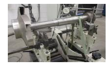
Once our processes are complete, all components undergo a final cleaning and quality control inspection. This process verifies that precision fits, running clearances, and shaft straightness meet or exceed OEM specifications. A careful assembly addresses radial and axial impeller position, thrust, and free rotation.
